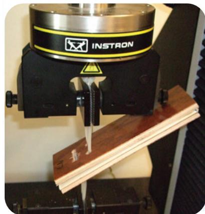
Lab tests show that the bond made with KOOL GLIDE® is more than 3 times stronger than with a finish nail.
