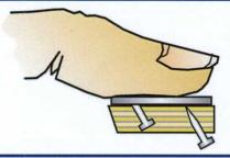
Lay the coin flat on the face of the strip where the pin has been removed and compare the width of the strip to the edges of the coin.
