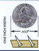
Lay the coin over the point of one of the pins in the strip to be measured.
