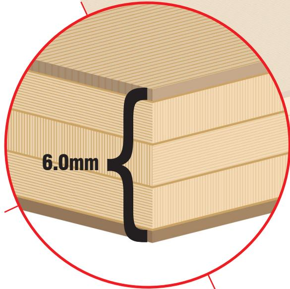
MasterPly™ Plywood Underlayment is constructed from 5 plies of premium hardwood veneers.
