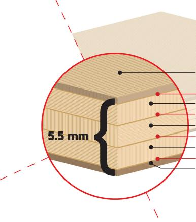
Top Pine Veneer Provides a Dense Smooth Surface. Sanded, Filled and Printed with Nailing Pattern
