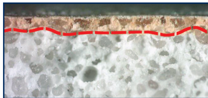
Petrography of freshly fractured cross-section of LIQUISHIELD 100™ treated slab. Beige-colored paste at the surface (above red line) repels water due to LIQUISHIELD 100™ penetration, while off-white paste not affected by the sealer (below red line) exhibits high water absorbency. Courtesy CTL Labs
