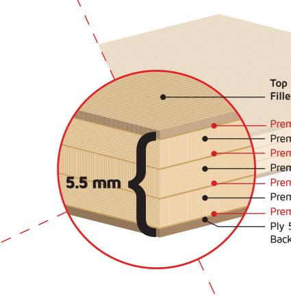
Top Veneer Provides a Dense Smooth Surface. Sanded, Filled and Printed with Nailing Patern
