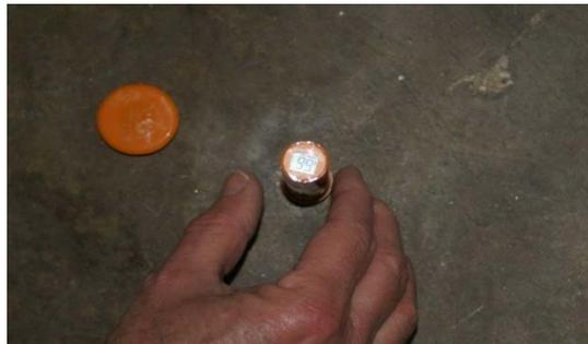
**\*\*\*TRAXXSHIELD99™ CAN BE USED UP TO A MAXIMUM READING OF 99.0% RH (PER THE ASTM F2170 STANDARD)\*\*\***
